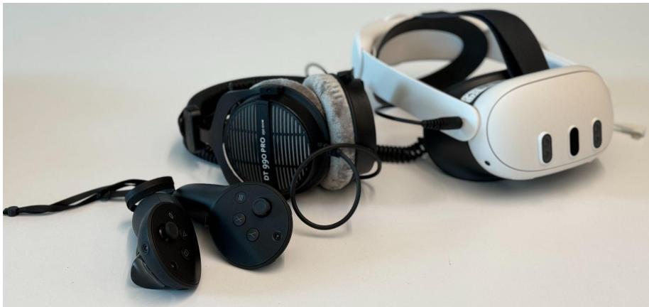
Figure 1. Equipment used during the sound localization test. From left to right: Quest Pro controllers, DT990 headphones, and Quest 3 headset with elite strap. During the experiment sounds were rendered through the Quest 3 headset, while participants were situated in VR and performed a localization task using the Quest Pro controllers.
